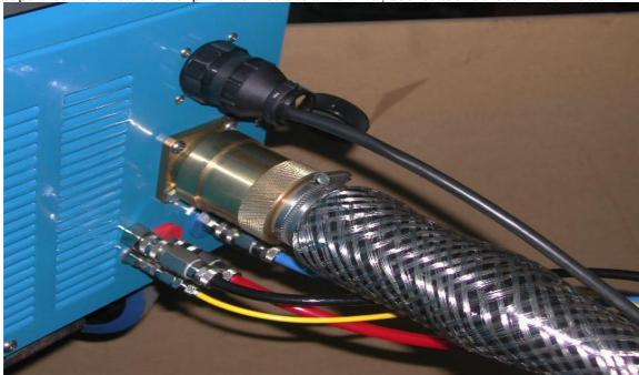
The two earth connectors (insert and twist clockwise to lock) are located on the left hand side of the front panel. An indicator lamp indicates when an earth loop has been successfully made.
