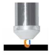
If the torch is pivoted about the nozzle there is a risk of material being blown back onto the nozzle which will cause damage to the nozzle or even to the torch itself.
